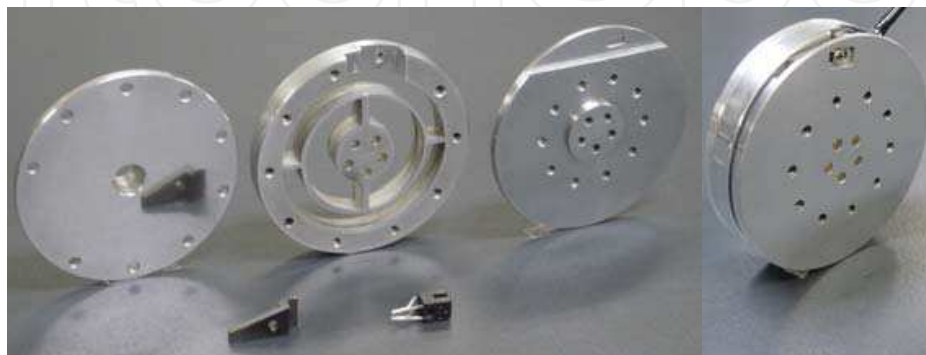
Fig. 12. Optical torque sensor with ring-shaped flexure
