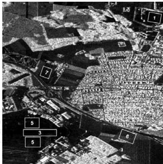
Fig. 1. Backscattered intensity image and regions of interest: [1] “water”, [2] “houses”, [3] “roads”, [4] “trees”, [5] “grass”, [6] “field 1”, [7] “field 2”.
