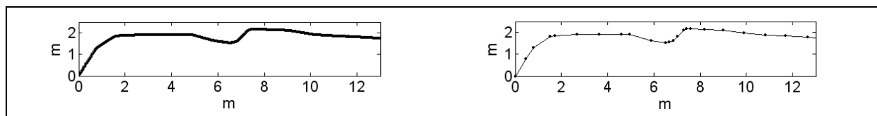
Fig. 5. Fragment of a real trajectory (left) and the polyline that approximates it (right). The dots represent the vertexes.
