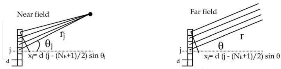
Fig. 18. Equally spaced linear array of hydrophone elements being intercepted by a propagating wave front at beam angles \theta_j for the near field configuration (left) with beam angle \theta for the far field (right) approximation.
