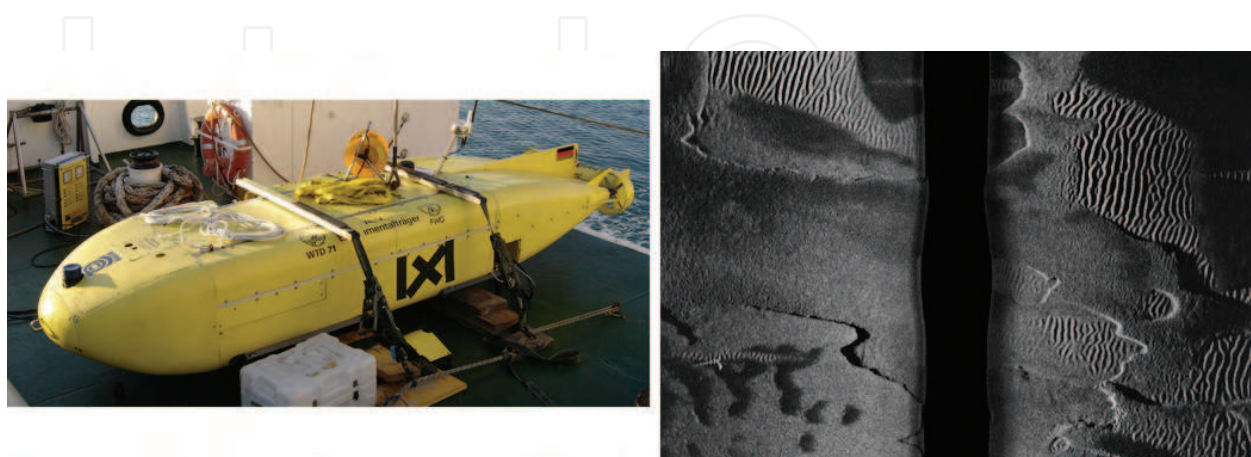
Fig. 5. The Sea Otter AUV and one of the images it collected during the MX3 trials with its Klein 2000 side-scan sonar.
