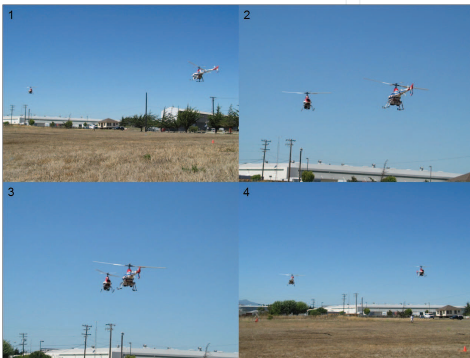
Figure 9. Mid-air collision avoidance between two rotorcraft UAVs using real-time MPC
