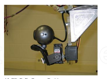
Figure 7. Quadrotor with Tilt-Roll Camera Positioner
