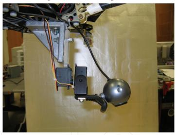
Figure 8. Quadrotor with Pan-Tilt Camera Positioner
