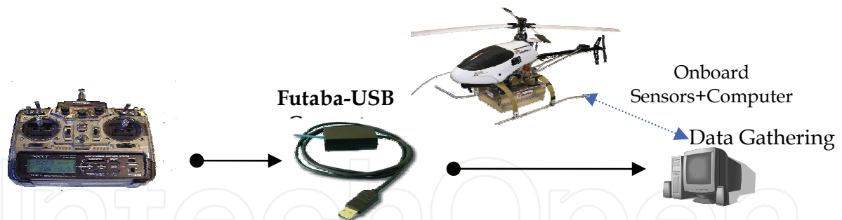
Figure 11. Data acquisition architecture
