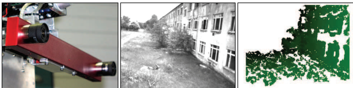
Figure 3. Stereo camera mounted at the helicopter (left), left onboard camera image (center), depth image (right)
