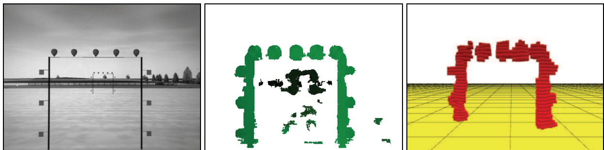
Figure 15. Original image from left camera (left), depth image (center) and extracted occupancy grid (right)
