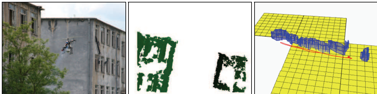
Figure 18. An urban environment (left), example of a depth image (center), and the resulting map (right) with obstacles, detected ground planes, and flight path
