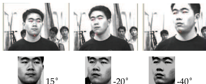
Fig. 6. Pose estimation results in surveillance system.
