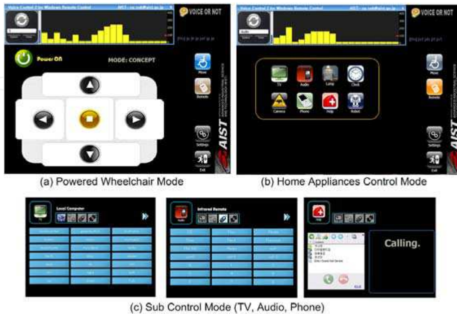
Fig. 7. Example of system GUI design (a) Powered wheel chair mode (b) Home appliances control mode (c) Appliance control sub mode
