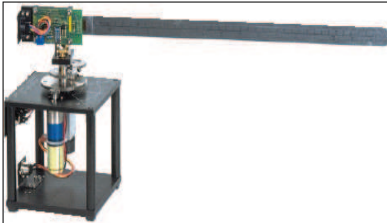
Fig. 2. Quanser Flexible Beam Experiment: SRV02-E servo plant and rotary flexible link module
