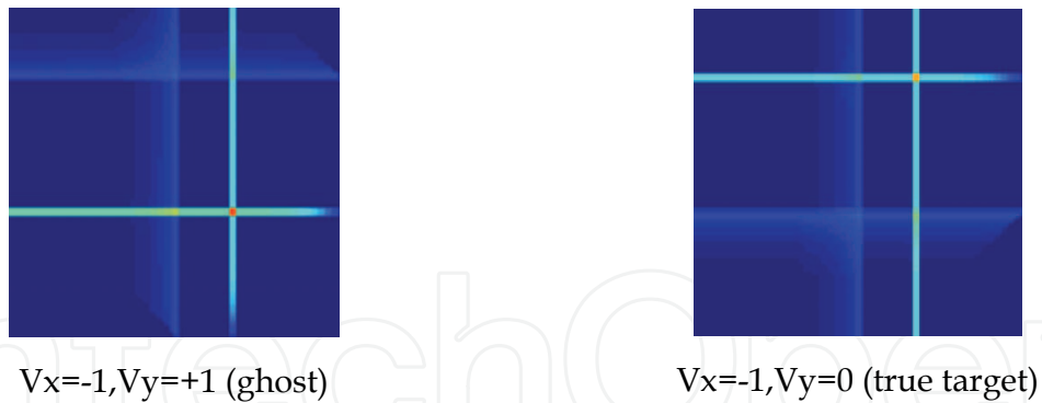
Fig. 17. Zoom of motion separated targets for time moment k=20
