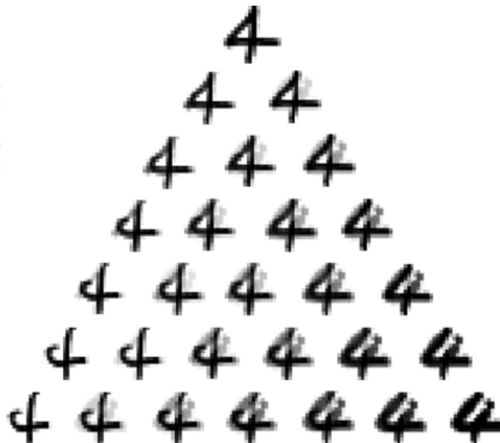
Fig. 2. A two-dimensional linear manifold spanned by three handwritten digit images '4' in the corners.
