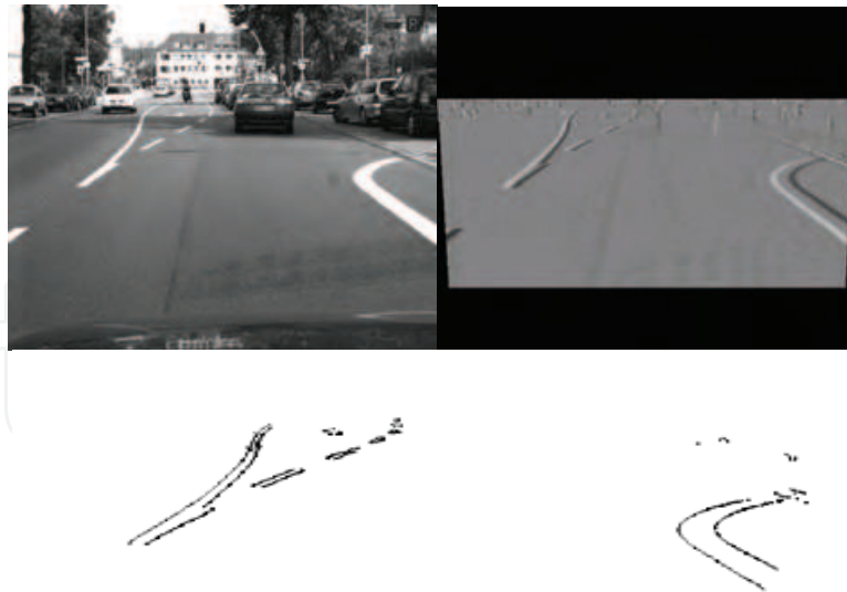
Fig. 4. Lane marking detection – top left, original image; top right, results of the adaptive gradient filter; bottom, lane marking results
