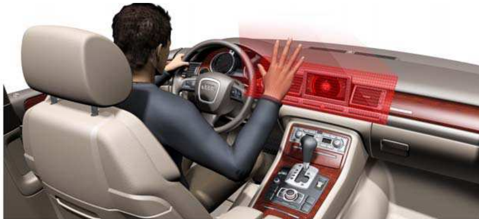
Fig. 4. Smart airbag application using a PMD TOF vision systems (Hussmann & Hess, 2006)
