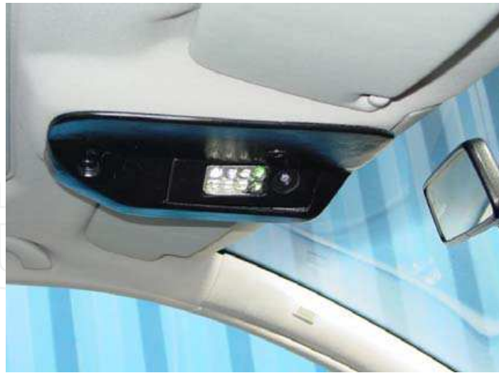
Fig. 4. Smart airbag application using a PMD TOF vision systems (Hussmann & Hess, 2006)
