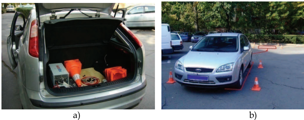
Fig. 9. The Ford Focus test vehicle; a) the DSpace Autobox in the carrier, connected to the CAN bus; b) a possible reference trajectory for a parking maneuver
