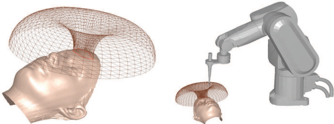
Fig. 5. Detail of a virtual shield and the scenario including the robot arm.
