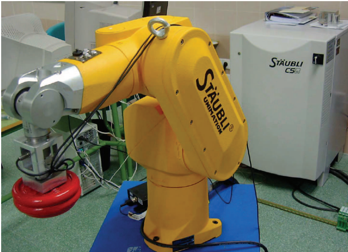
Figure 4. Stäubli Platform. An RX60 robot with an open control architecture system is used. An ATI wrist force sensor is attached to the robot tip. The accelerometer is placed between the robot TCP and the force sensor
