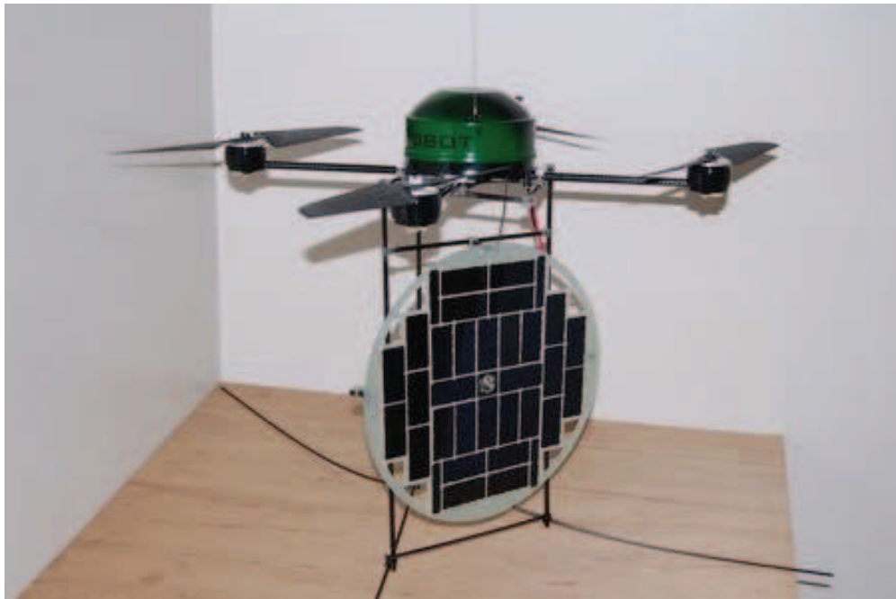
Fig. 8. Helicopter with a vertical solar panel underneath
