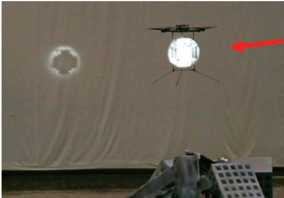
Fig. 9. Helicopter flight receiving the energy from the laser energy transmission over a simulated disaster ruin
