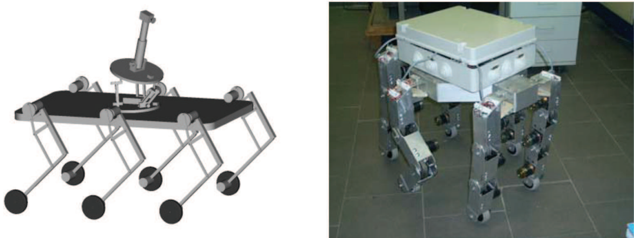
Fig. 15. The Cassino hexapod robot for Survey activity as a general kinematic scheme and a built prototype.
