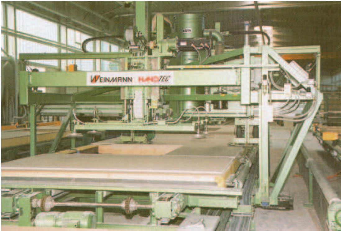
Fig. 5. Multifunctional robotic wooden wall production unit
