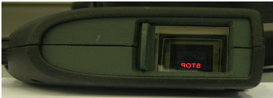
Fig.3. "Stop" signal displayed on the external side of LITEYE-500 eyepiece
