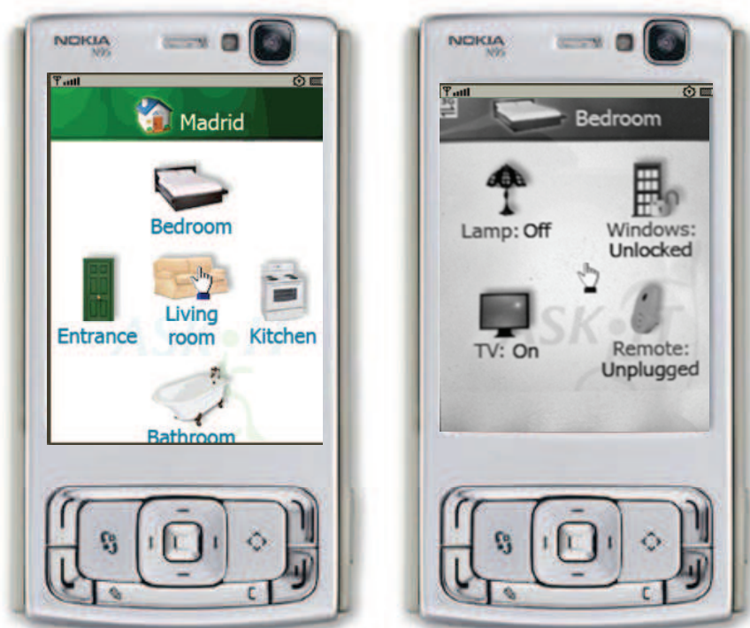
Figure 4. Domotics UI for a Smart Phone (left). UI adapted to a visually impaired user, indicating the status of several devices in the bedroom (right)
