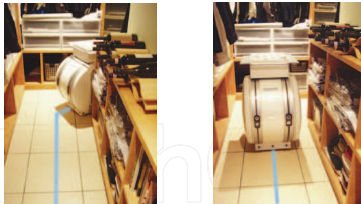
Fig. 8. Robot in movement, guided by line-marker
