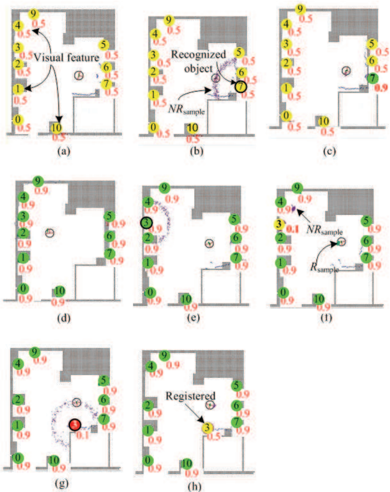
Fig. 10. Experimental results; (a), (b), (c) and (d) are procedure of increasing reliability of pose, (e),(f),(g) and (h) are procedure of intelligent update of visual map.
