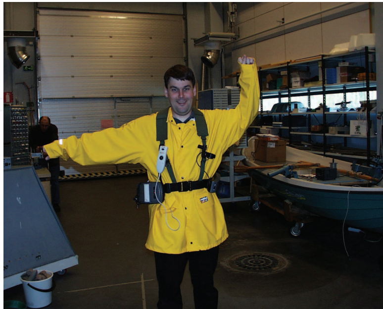
Fig. 10. Use of gestures in commanding. Gestures are recognized by the robot's camera head, which tracks the colored jacket of the user.
