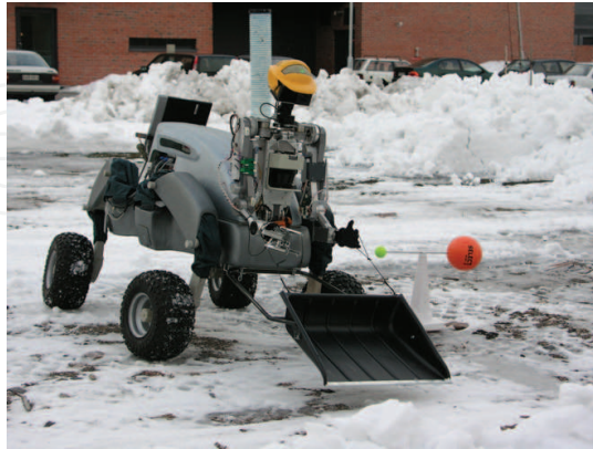
Fig. 3. WorkPartner service robot cleaning snow from the yard
