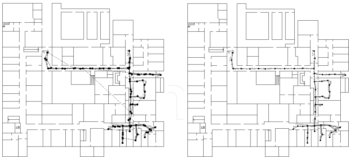
Figures 11 (left) and 12 (right). Left: topological loop closing, accepted hypotheses are shown in thick black lines, rejected in dashed thin black lines. Right: the resulting topological map, locations of the place prototypes with interconnections
