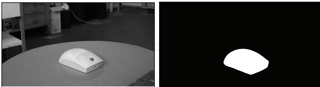
Figure 15. A computer mouse: the object acquired image (left), the computed object silhouette region (right)
