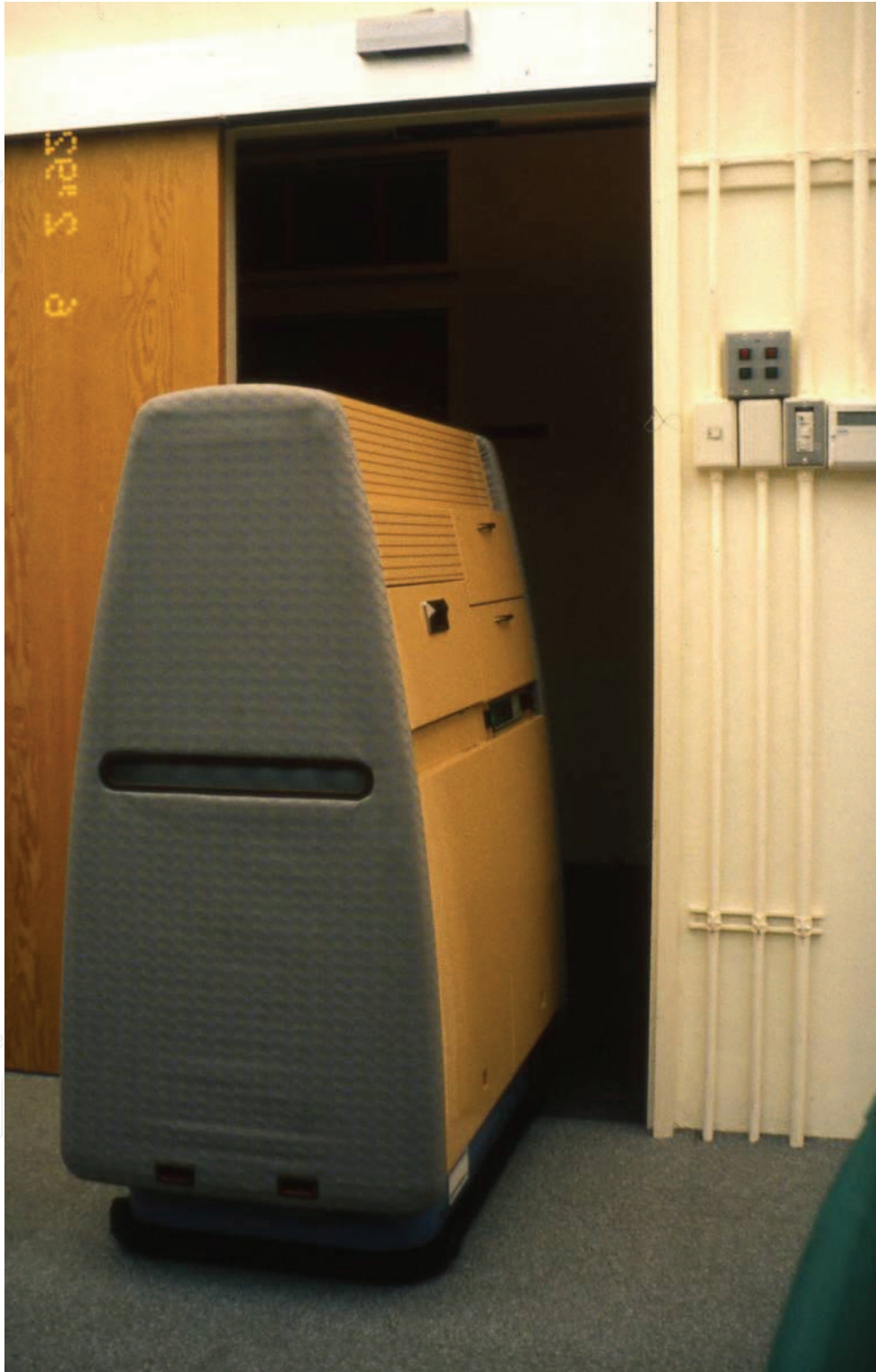
Fig. 4 Tron office service robot
