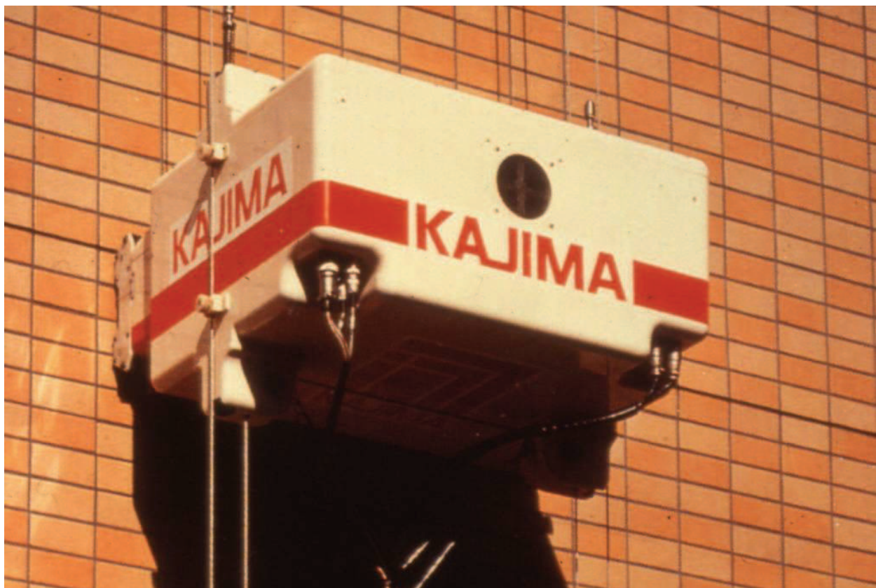
Fig.1 Kajima façade diagnostic robot
