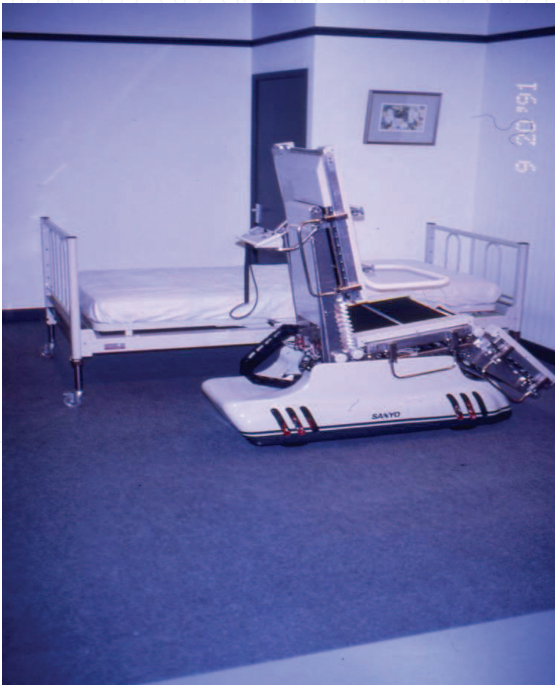
Fig. 10 Sanyo robotic patient transfer and wheelchair System
