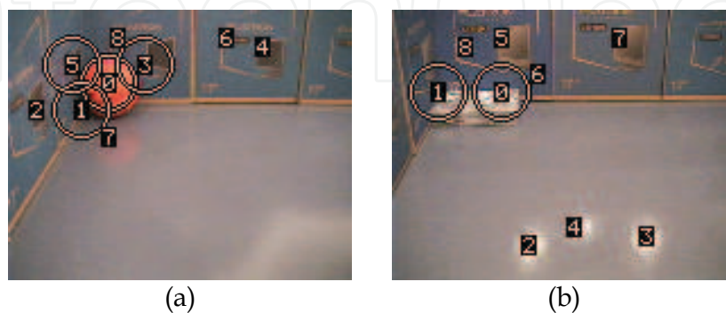
Figure 8. Examples of output images for the laboratory experiments: (a) orange ball (GWR and PCA); (b) grey box (GWR and PCA). The numbers indicate the location of salient points in order of importance (0 corresponds to the most salient) and the white circles indicate that the region corresponding to a particular salient point was labelled as novel.
