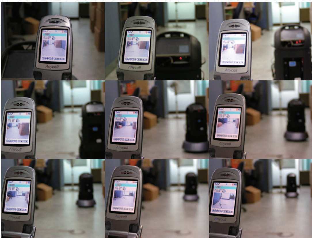
Fig. 10. Images transmitted to mobile robot as SG-Robot moves.
