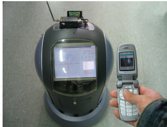
Fig. 8. Operation of SG-Robot using mobile phone.
