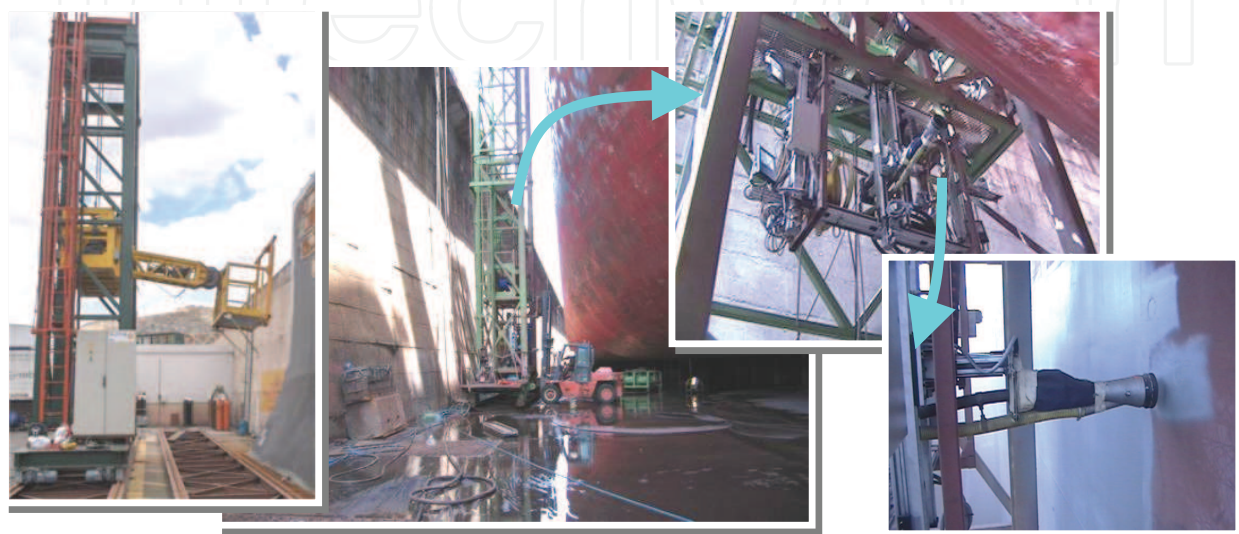
Fig. 3. Crane robot for cleaning vertical surfaces in EFTCoR.
