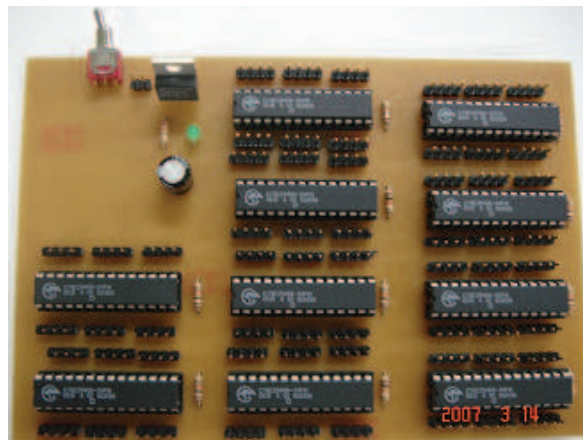
Fig. 16. Photo of the proposed distributed PSoC based controller.
