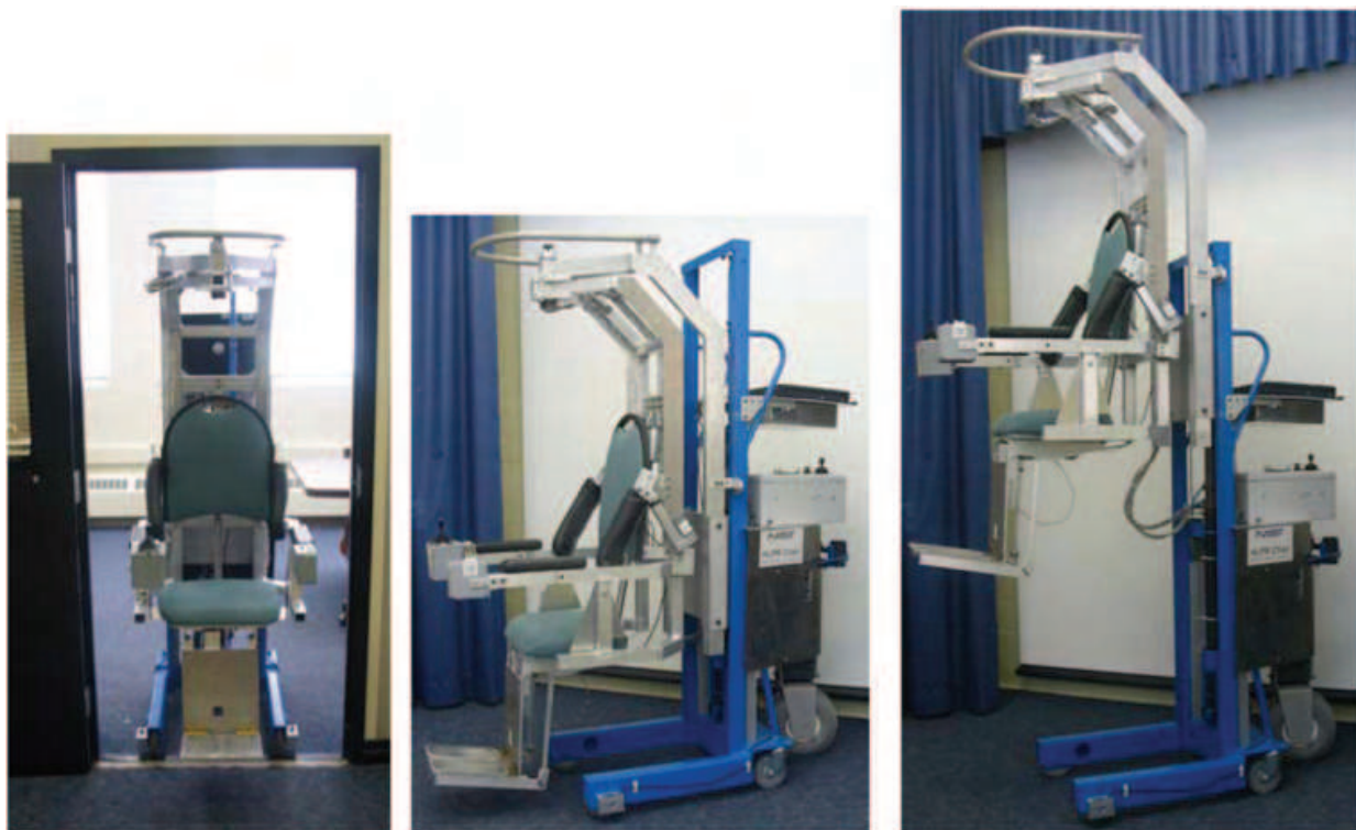
Fig. 6. The HLPR Chair in the mobility configuration showing the front view relative to a typical doorway (left), the side view (center) and the patient lift position (right).
