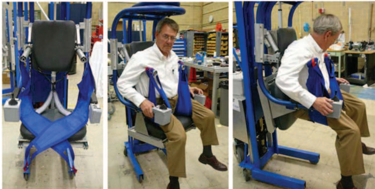
Fig. 14. Photographs of the HLPR Chair sling showing (left) the sling ready for the patient to be seated, (center) a patient with the sling ready to lift while seated on the HLPR Chair seat, and (right) the patient fully supported by the sling with the HLPR Chair seat rotated behind the patient.
