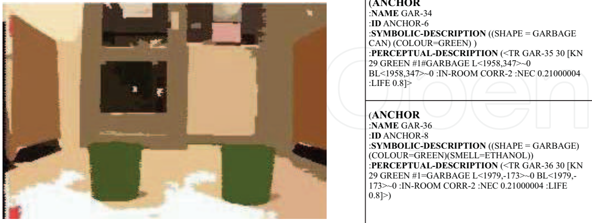
Fig. 3. (Left) Segmented image from the vision module observing two green garbage cans at the center of the screen. (Right) The anchors created in a bottom-up manner for each object. Gar-34 refers to the garbage can on the left of the image and Gar-36 refers to the garbage can on the right.
