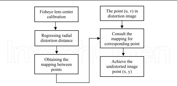
Fig. 3. Flow chart of fisheye image restoration algorithm
