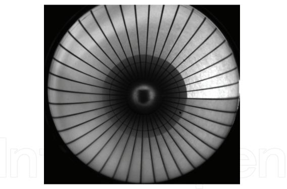
Fig. 1. Radial straight lines in fisheye lens image under cylinder model
