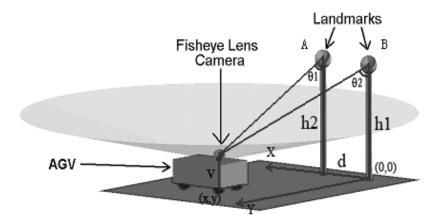
Fig. 6. Physical space coordinates system for landmarks localization
