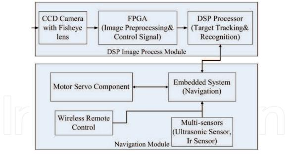
Fig. 9. Hardware configuration of the unique navigator
