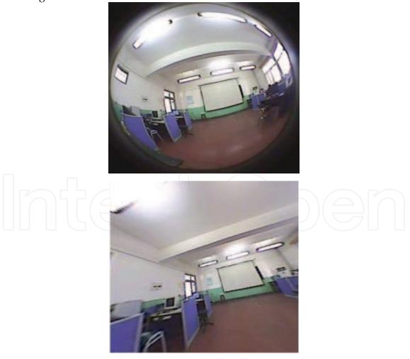
Fig. 4. A fisheye image (above) and the corrected result of a fisheye image (below)
