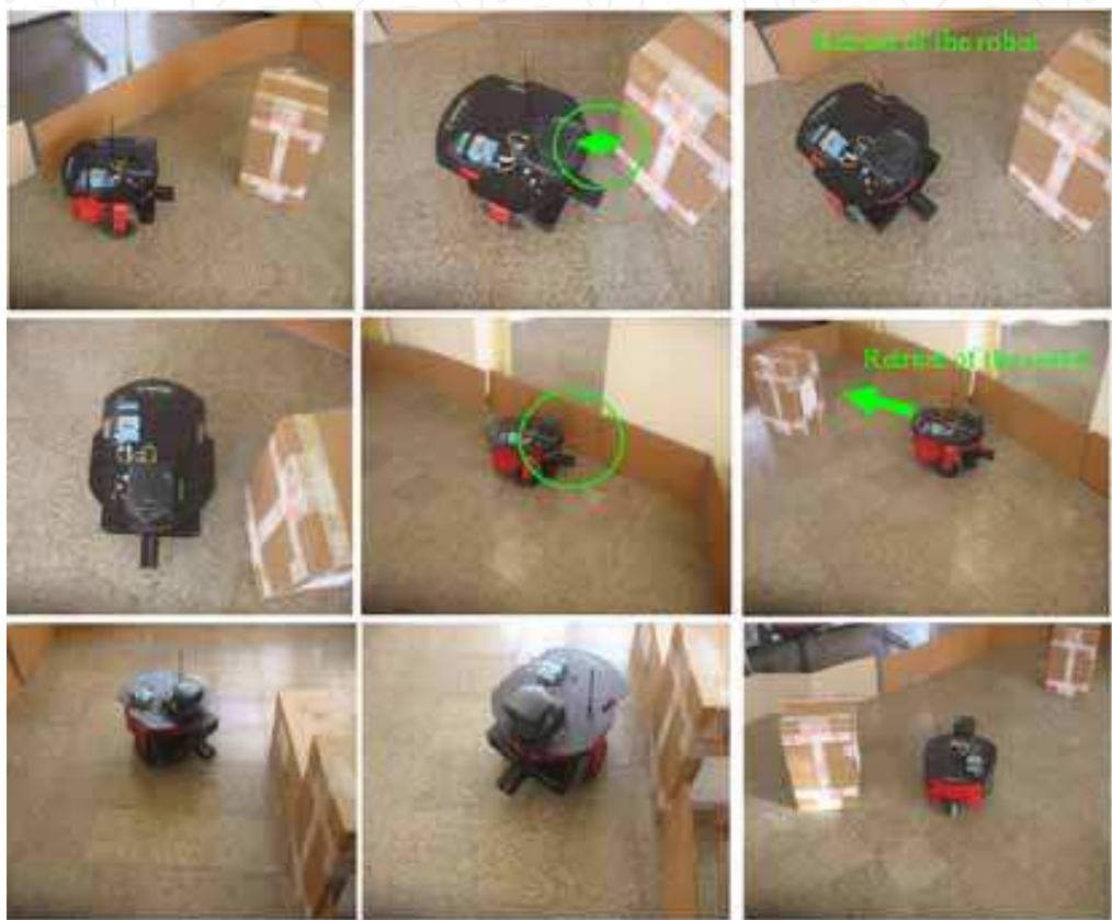
Fig. 13. On line learning of the real robot Pioneer II, behaviour "Obstacle Avoidance»
