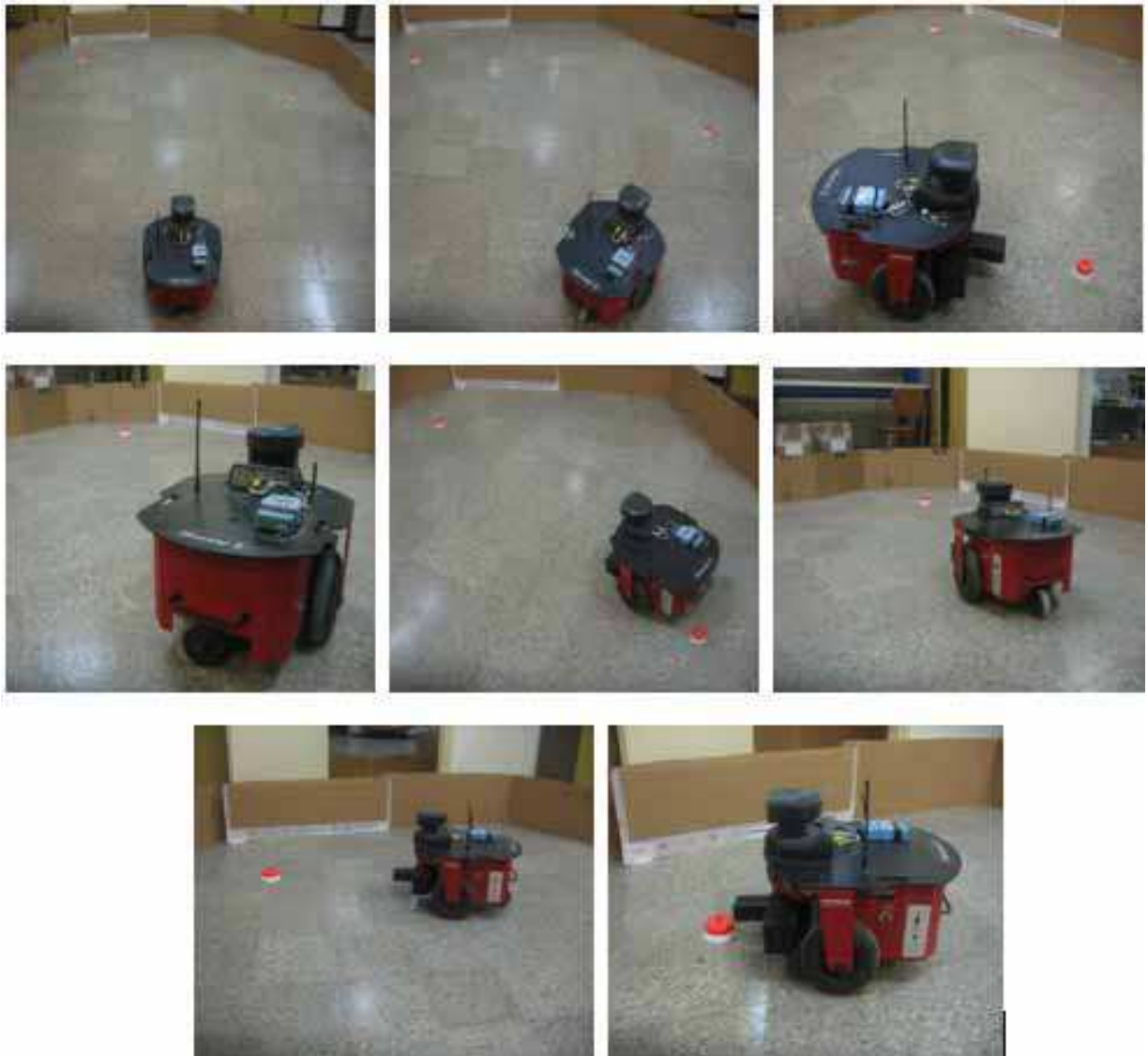
Fig. 32. Validation of the FIS obtained in simulation by algorithm DFQLGA on the real robot Pioneer II for the “Go to goal” behaviour
