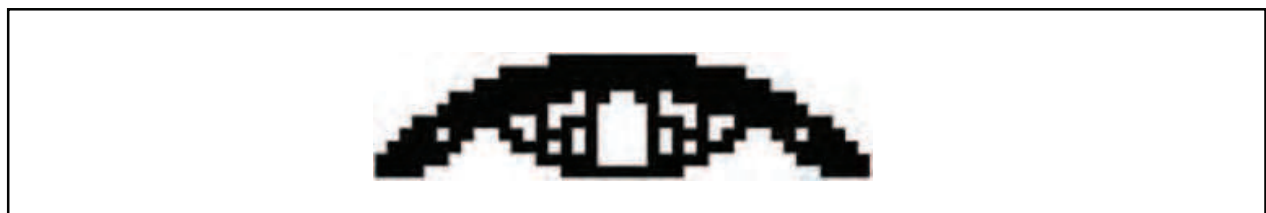
Fig. 27. Optimal topology of the MBB beam (Bureerat & Kunakote, 2006).
