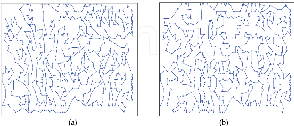
Fig. 7. Solutions found to u724 data. (a) Feasible solution found without local search improvement with 469 epochs and average error of 16.85%. (b) Feasible solution found with local search improvement with 516 epochs and average error of 6.28%.
