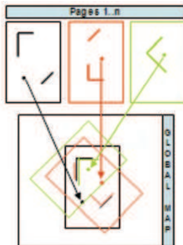
Figure 4. Single scans are transformed to build a global map
