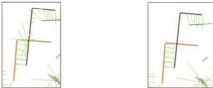
Figure 6. Left: forces between two scans (red lines belong to first scan, black lines to second scan) computed without direction information. Right: forces computed using L and K as described in example 2 (using equal masses). Correspondences between non parallel structures are weakened
