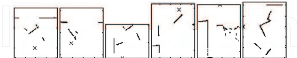
Figure 8. 6 out of 60 scans of the NIST rescue scenario data set. The scans in this data set are very sparse and have minimal overlap
