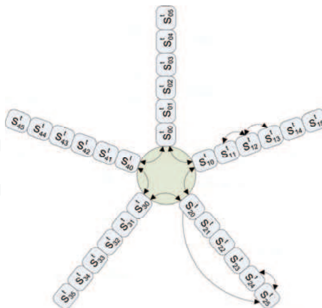
Figure 8. The two-dimensional CA lattice. The arrows represent the interaction between a cell (possibly located somewhere in the middle or on the edge of the lattice) and its neighboring cells. Essentially the interaction is similar to the model in §3.2 except modules closest to central disc interact with modules in similar position located on the neighboring leg
