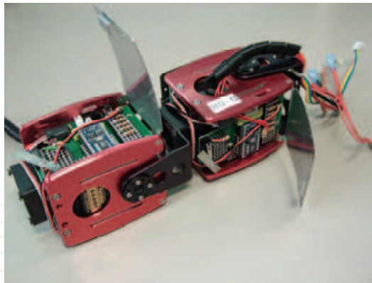
Figure 3. Exposed view of adjacent connected modules
