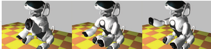
Figure 16. Sequence of the oscillation obtained in simulation for the J1 joint type. The robot is sit on its butt to allow a free movement of the joint. The evolution of the other joint types was performed with the same setup and similar behaviors were observed
