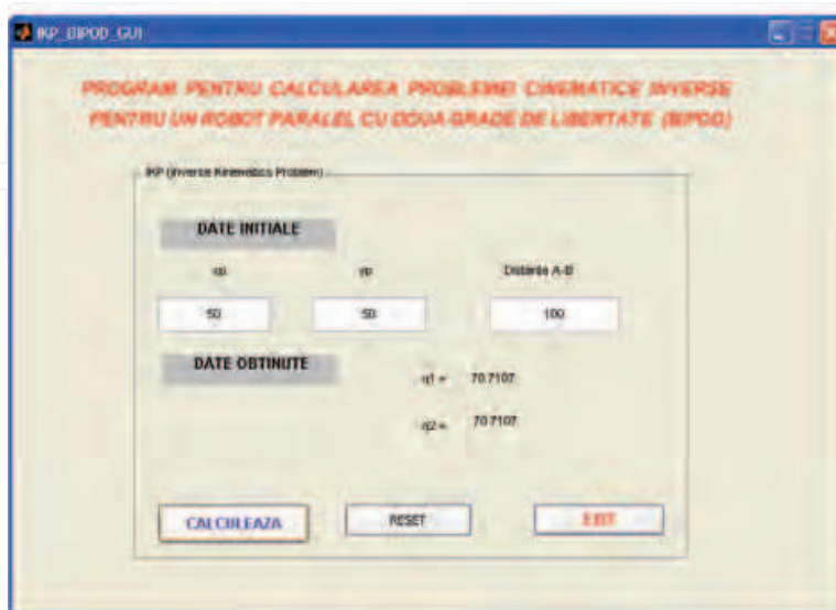
Fig. 8. Graphical User Interface (GUI) for solving inverse kinematics of the 2 DOF planar Parallel Kinematics Machine of type Bipod in MATLAB environment.
