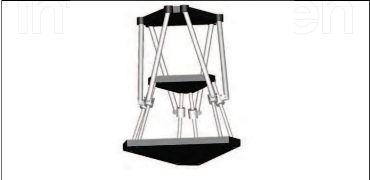
Fig. 1. New hexapod design
