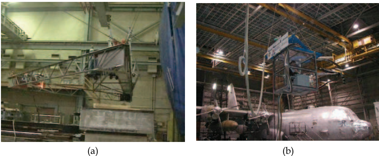
Fig. 3. The NIST Flying Carpet – a platform for ship access in drydocks (a) and the NIST Aircraft Maintenance Project (AMP) – a platform for aircraft access in hangars (b).
