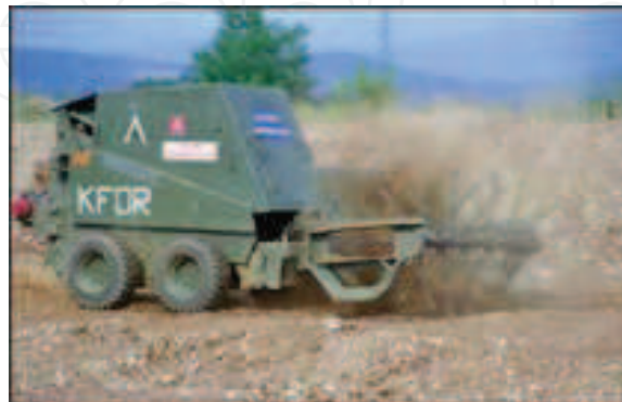
Fig. 1. The remotely operated flailing vehicle “Božena 1”
