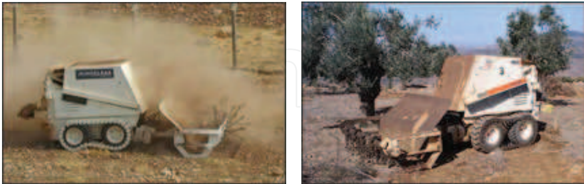
Fig. 2. The mini-flail vehicles “Božena 2 and 3”
