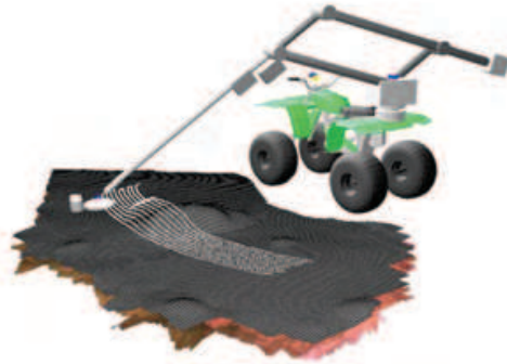
Fig. 11. Environment modelled with the stereo vision camera
