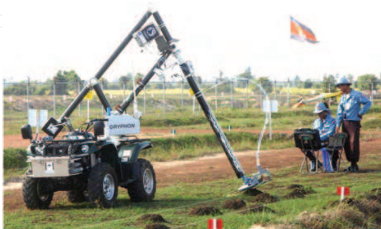
Fig. 12. Gryphon autonomously scanning a test minefield in Cambodia under the supervision of Cambodian deminers
