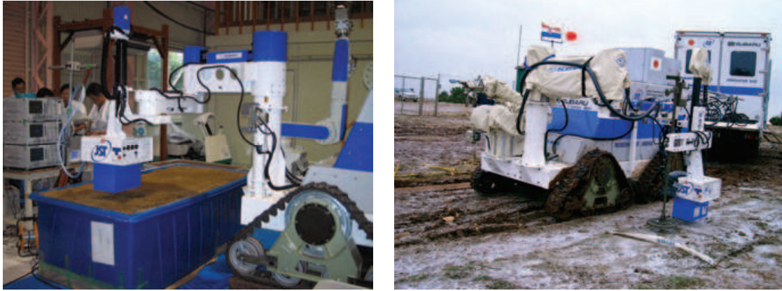
(a) SAR-GPR mounted on a robotic arm and scans in front of the MHV. (b) SAR-GPR in operation in CROMAC test site. SAR-GPR scans in the side of MHV
