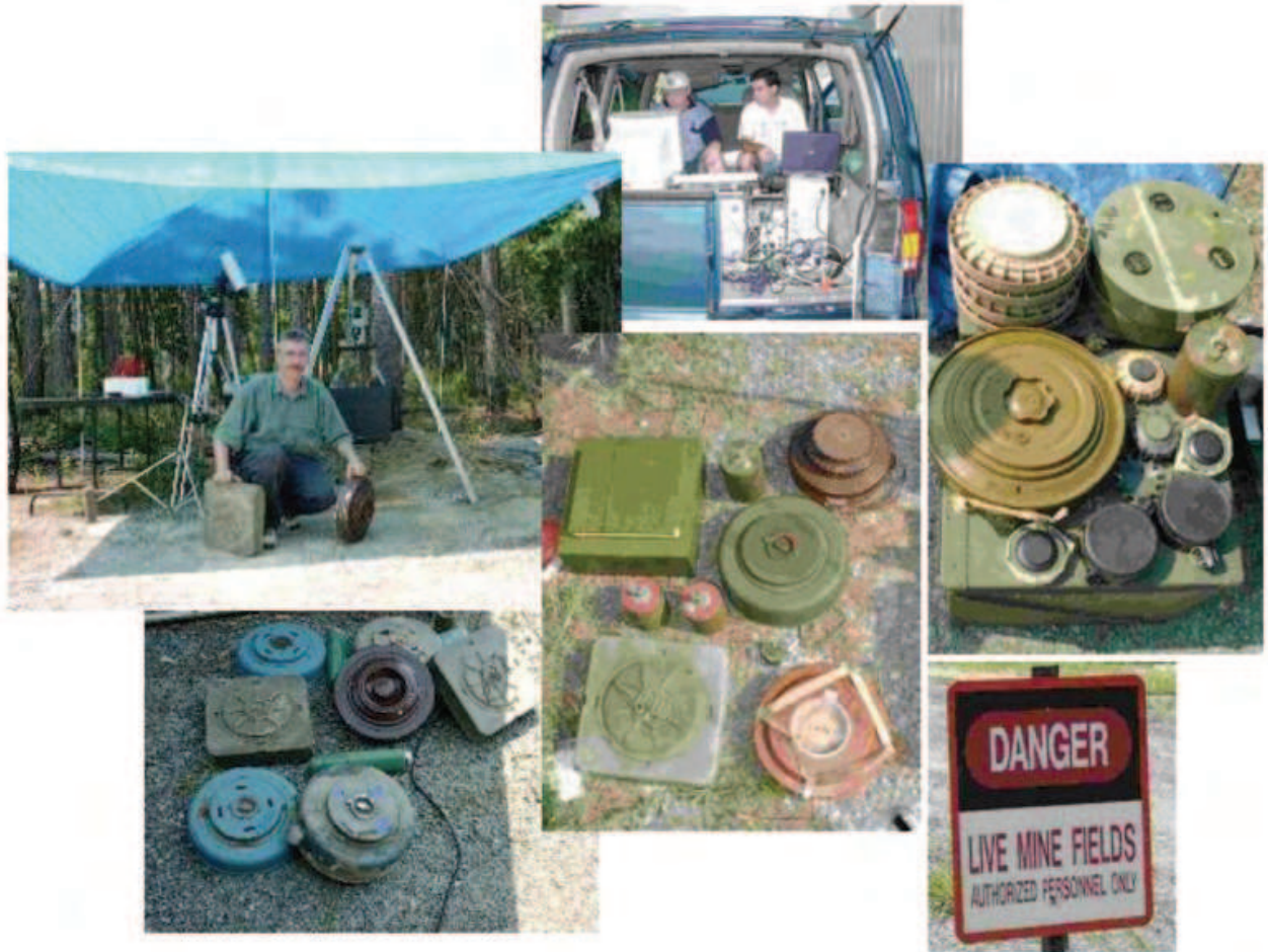
Fig. 2. Collection of live mines and experimental setup for dynamic impedance measurements of mines at U.S. Army testing ground
