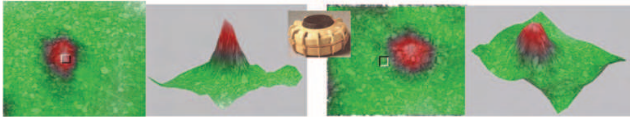
Fig. 24. Nonlinear images of AP mine VS-50 buried in gravel at 12 mm (left), NDC =19dB, and 25 mm (right), NDC =16dB
